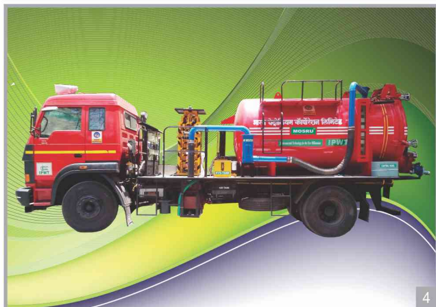
4. Mid-size MOSRU ® (6000 lbs.) ; on 16 ton GVW chassis ; supplied to Bharat Petroleum Corporation Limited, Mahul Refinery in 2014.
